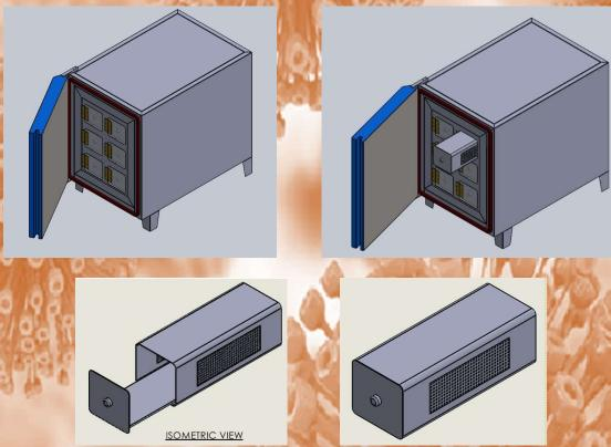
Cell Locker with Stainless Steel Tray, Stainless Steel, Dual 0.2µm membrane filters
